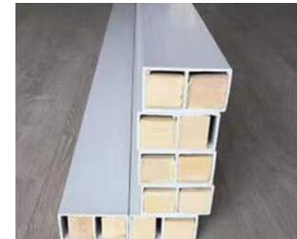
2. Fix the bottom of the tubes by putting the wood blocks in the tubes and then fixing the blocks and tube together by nail-free adhesive.
